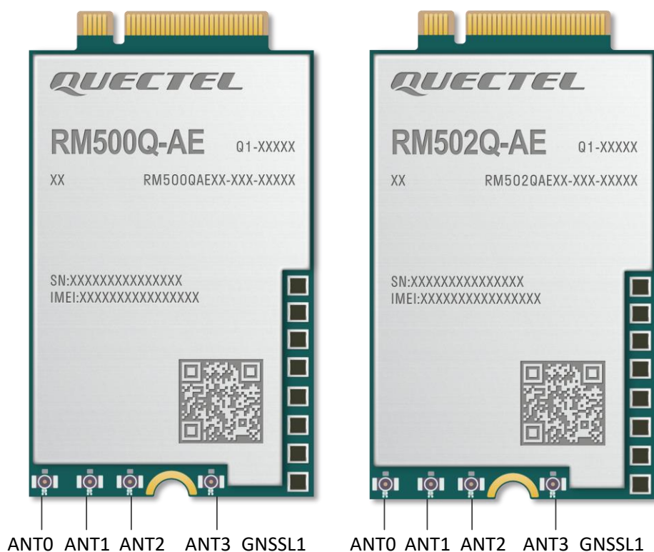
Figure 27: Antenna Connectors on RM500Q-AE & RM502Q-AE
